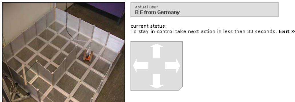
Fig. 2. RCL „Robot in a Maze“: the variable maze and the robot vehicle are seen on the left. Two viewing modes are possible: tilted laboratory view from above (image left) and robot view (web cam placed on the robot). The relatively simple controls of the robot and the status display are visible on the right hand side.
