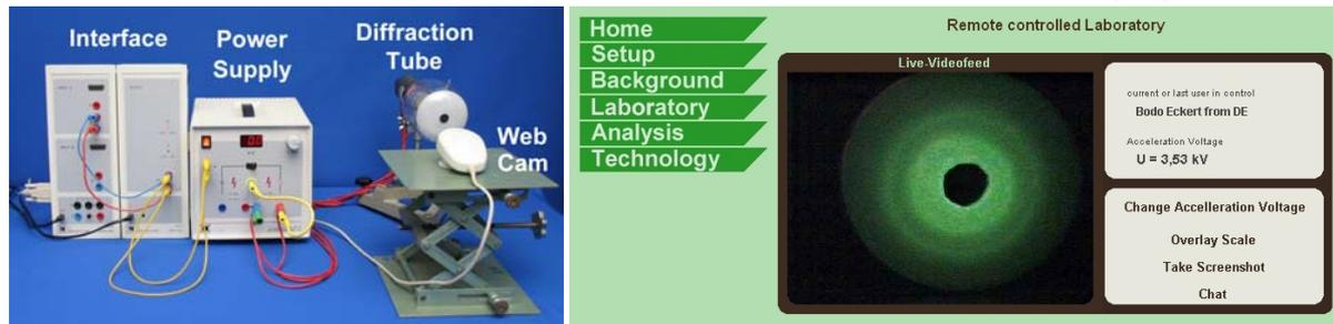
**Fig. 3.** RCL „Electron Diffraction Tube“: set up of the experiment with CASSY-interface, power supply, electron tube and web cam (left). Part of the website under option „Laboratory“: live video stream (the diffraction order 0 is blocked) as well as chosen acceleration voltage and voluntary user data (right).
